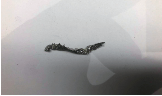
图10 CFRP/Ti叠层钻削过程中的钛合金切屑 Fig.10 Titanium alloy chip in CFRP/Ti drilling
